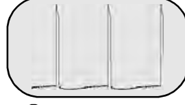
⑩ 30.4 Vp-p IC451 PIN 3 (PUMP UP)
